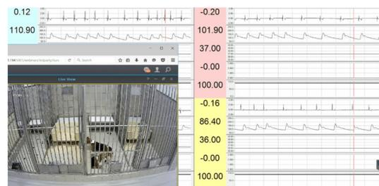
Electrocardiogram and blood pressure recorded from implanted dogs using emka TECHNOLOGIES easyTEL+ implants.
