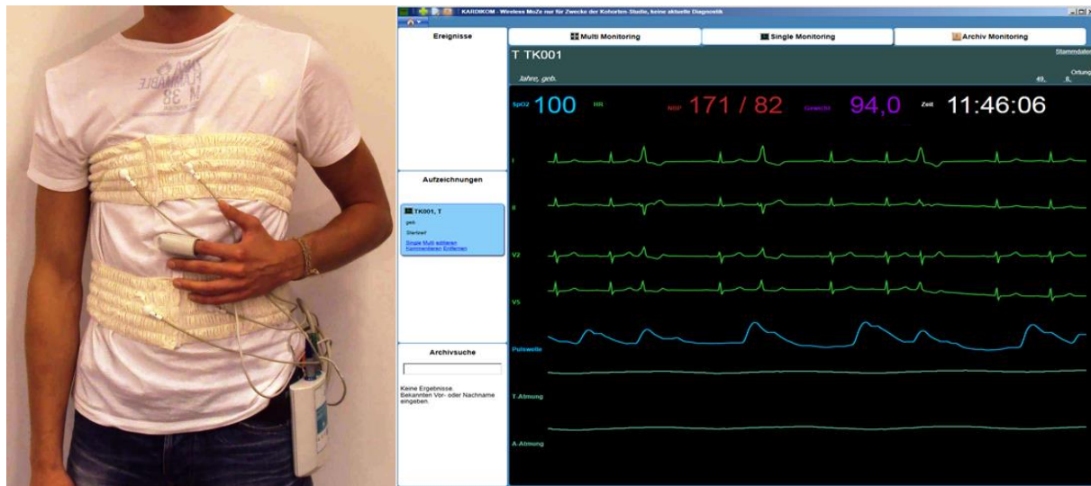
Figure 2a & b: The left picture illustrates the application of the wireless data logger system “Cor/log® BAN BT”. The person carries the “Cor/log® BAN BT” on his left hip. The following sensors are visible: the two breathing belts, one around the thorax and one around the abdomen and the pulse oximeter on the left index finger. The ECG electrodes are attached underneath the shirt. Figure 2b: The right picture is a screen shot of the almost realtime telemedical monitoring software. The software displays the following physiological parameters in numbers: SpO 2 in blue; heart rate in green; blood pressure in red, and weight in purple (pressure and weight from external devices). The following physiological vital sign waveforms displayed from top to bottom are: ECG in green, SpO 2 photoplethysmogram in blue and two respiration belt waves in cyan.
